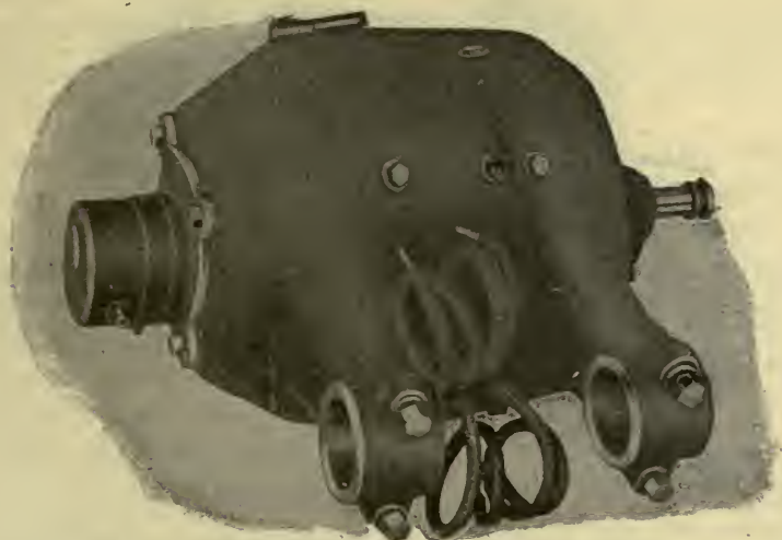
FIG. 423.—General Electric Motor, Designed for Heavy Vehicle Use, with single or double reduction. Capacity, 30 amperes at 85 volts; 800 R. P. M. at full load.
